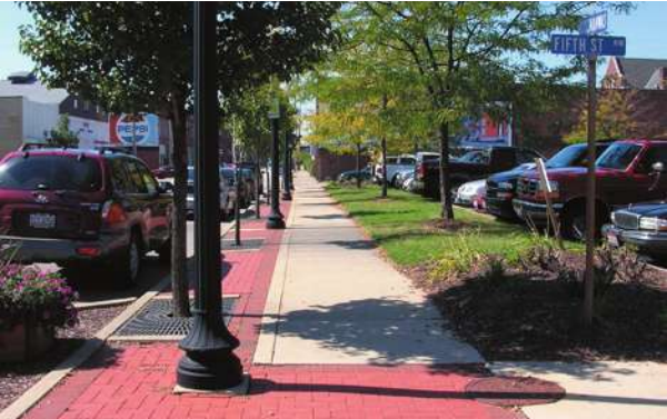
Downtown Barberton, Tuscarawas Avenue showing street trees and on-street parking between the pedestrian sidewalk and the roadway, a tree lawn separating a parking lot from the sidewalk and other amenities like light poles and a brick paver curbwalk with street tree planters.
